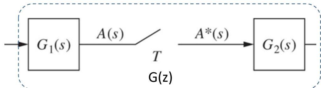
$$G(z) = Z(G_1(s))Z(G_2(s)) = G_1(z) G_2(z) \quad \checkmark$$
