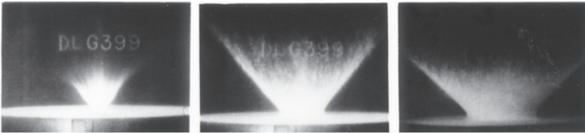
Figure 6.29 The excavation flow forms an outward expanding conical ejecta curtain. The excavation flow in a large planetary impact is thought to be very similar to that from this small impact in a laboratory. (Courtesy P.H. Schultz)
