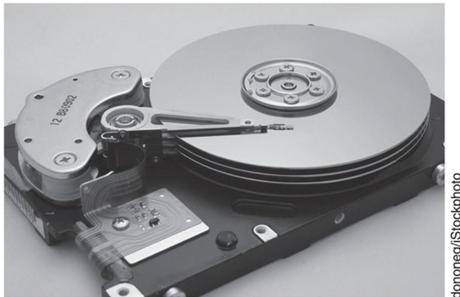
FIGURE 1.6 Computer hard disk drive, showing disks and read/write head
