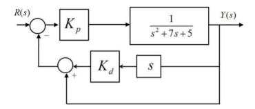
Using the properties of second-order systems, determine  $K_p$  and  $K_d$  such that the overshoot is 10 percent and the settling time is 1 second. Confirm that your design meets the requirements by plotting the step response in Matlab.
