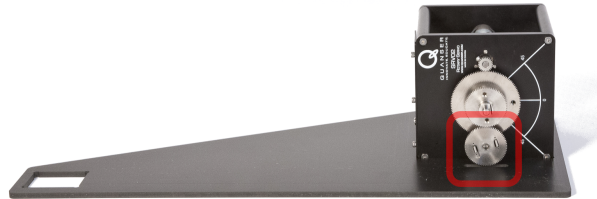
Figure 4.1: Place SRV02 in calibration base
