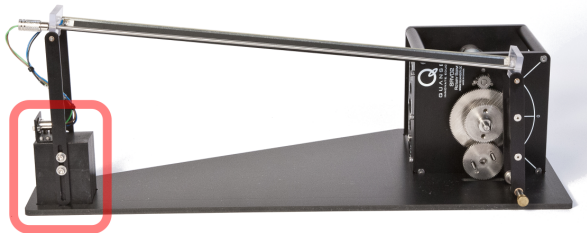
Figure 4.2: Place BB01 support column in calibration base
