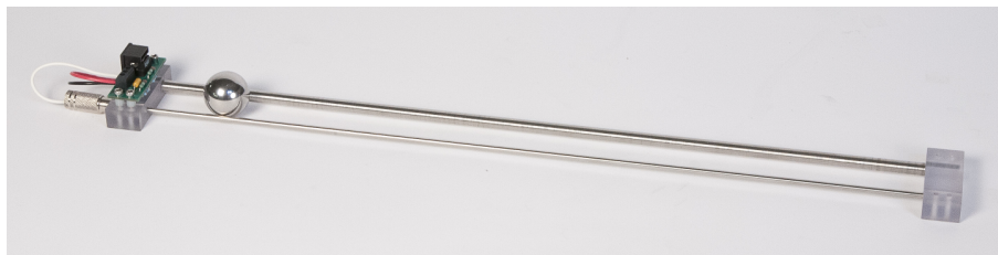
Figure 1.2: Quanser Remote Sensor (SS01) system
